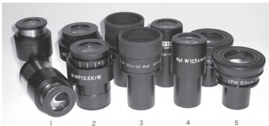
図5 接眼レンズ。— 1: Leitz W 6.3×/28 (φ30.0 mm), 2: Motic N-WF 12.5×/18 (φ30.0 mm), 3: Leitz GF 12.5×/20 (φ23.2 mm), 4: Zeiss kpl W 12.5/18 (φ23.2 mm), 5: Nikon CFW 12.5×/16 (φ23.2 mm),
